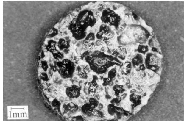
Figure 2 Optical micrograph showing the macro and micropores of the inner part of the composite where gelatin (blue colored by genipin) fills the inner part of the pores.
